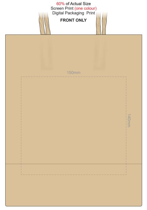
Digital Packaging Print is only available on white and natural products. As this is an uncoated substrate and artwork is printed directly onto the product via CMYK print with no white ink base, ink is absorbed into the product, giving the artwork a faded, vintage finish.
